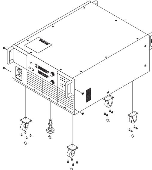
2. As shown in figure, using the accompanying screws, install the brackets.
